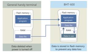
• Inputted data is saved in the terminal's flash memory, preventing data loss even when the battery runs out of power.
