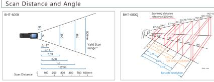
\*\*Laser beam amplitude is approximately 90% of the decode range (including margin). 40, 200, 450, 500 are the valid scan range from each distance.
